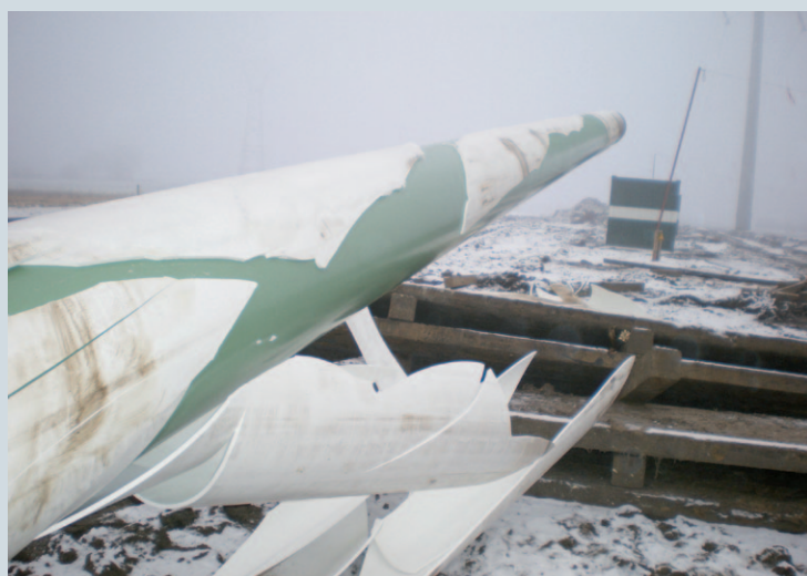
FIGURE 1 AND FIGURE 2: PP coating damage discovered on a buried pipe and pipes on stock
