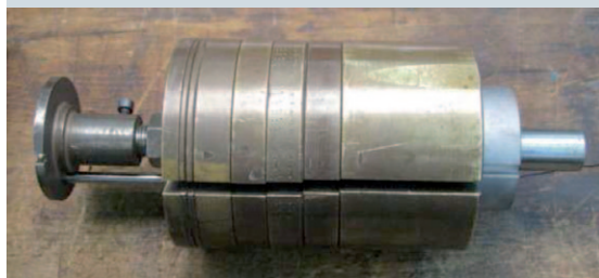
FIGURE 4: Drop weight used for modified impact testing
