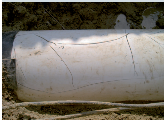
FIGURE 10: Cracking pattern as produced by low-temperature embrittlement
