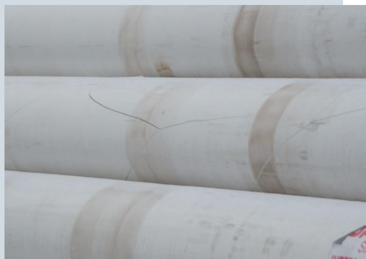
FIGURE 1 AND FIGURE 2: PP coating damage discovered on a buried pipe and pipes on stock
