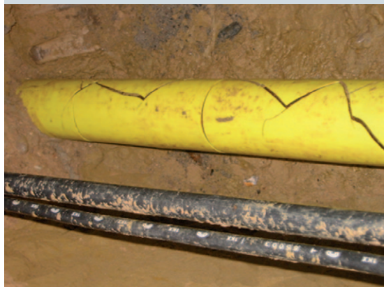
FIGURE 9: Cracking pattern as produced by aging of the material
